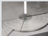
Round supporting table The machine has a supporting table that rotates along with mitre cuts. This means that there are no recesses
