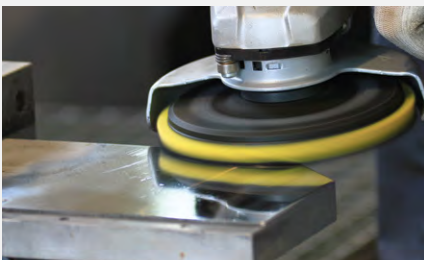
Subsequent mirror finish polish with the BRIGHTEX® polishing system (Berry + Sun). See the polishing section starting on page 214.
