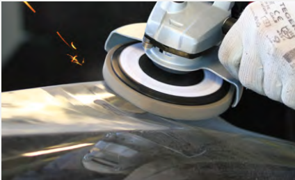
Removes scratches and small spot welds and seams all at the same time.
