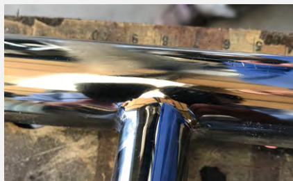
Result: raw to perfect mirror finish in two to three steps – also ideal for round pipes.
